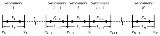
**Figure 4**: Variable definitions for models. F is the sarcomere force produced from the ith sarcomere, L is the length of the ith sarcomere, and x is the total distance of the ith sarcomere from the start of the myofibril.
