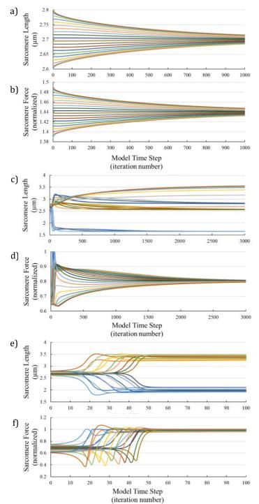
**Figure 7:** Simulation results for twenty dependent sarcomeres with passive force shifting to the right with constants C = 0.1 with sarcomere lengths (a) and forces (b) over time, C = 0.2 with sarcomere lengths (c) and forces (d) over tine, C=0.3, with sarcomere lengths (e) and forces over time (f).
