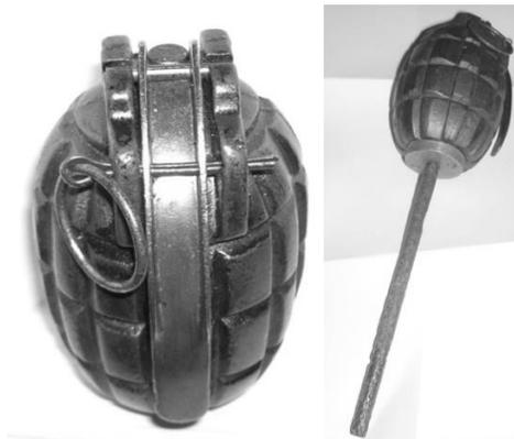
Mills No. 5 hand grenade and Mills No. 23 rifle grenade used by the Canadian Corps with rod attached.
